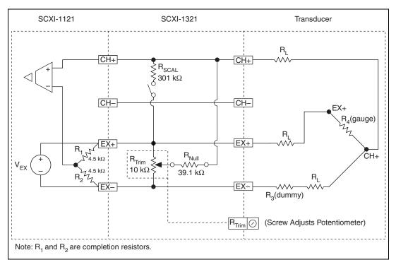
Figure 3. Quarter-Bridge Nulling Circuit
